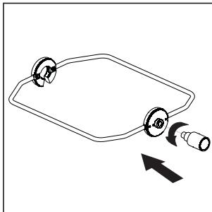
Screw the corresponding adapter into the bar frame base from below:
